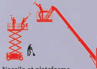
Nacelle et plateforme Boom lift and Scissor lift
