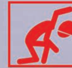
Espace clos Confined Space
